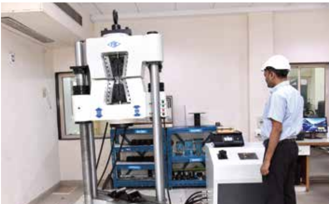
Universal Testing Machine, UTM-2 capacity: 1000Tones
